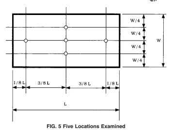
viewed surface. Place the spandrel glass sample against an opaque backup material and in a vertical position. View the sample from a distance of approximately 3 m (10 ft). Determine acceptability in accordance with 8.3.1.
