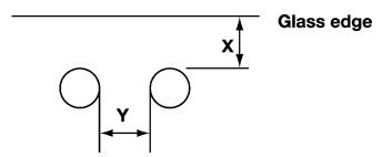
X = 6 mm ( $\frac{1}{4}$  in.) or 2t, whichever is greater Y = 10 mm ( $\frac{3}{6}$  in.) or 2t, whichever is greater Where:
