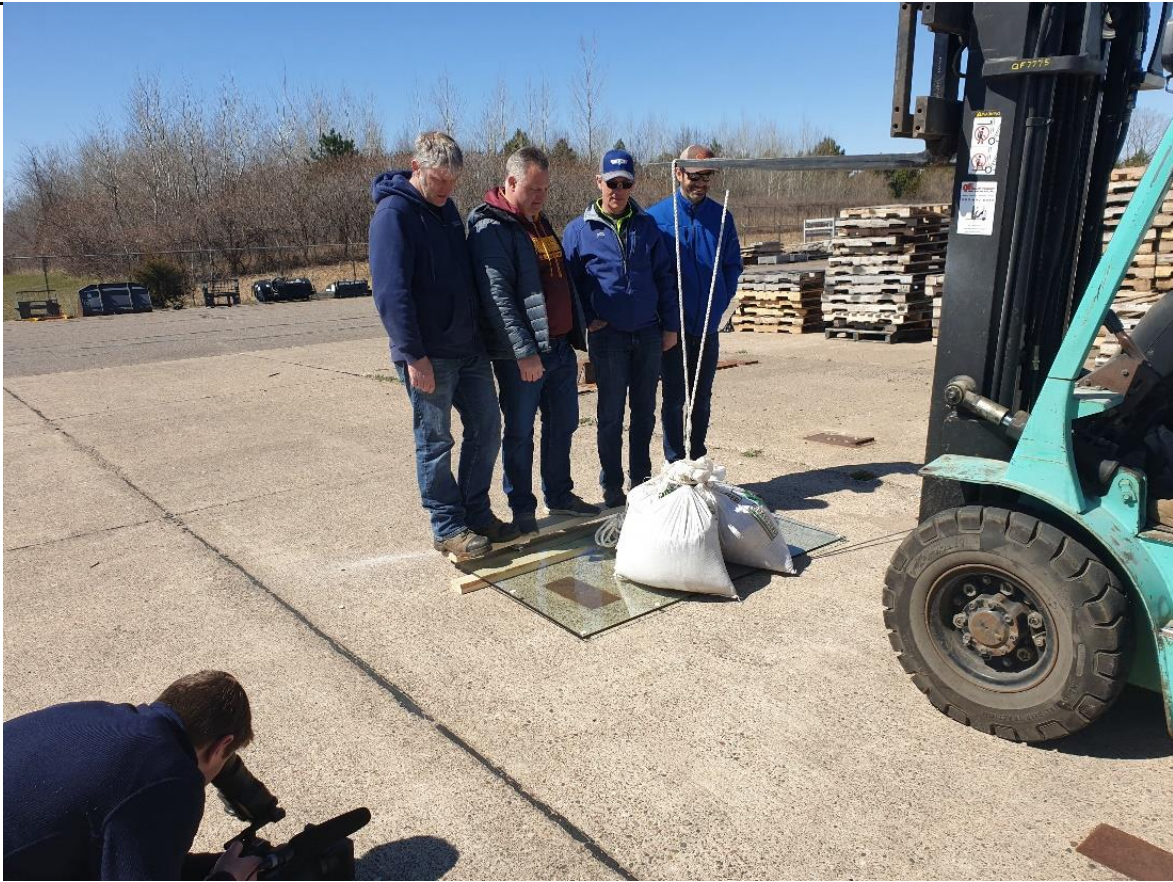
Photo 5: Horizontal load test
