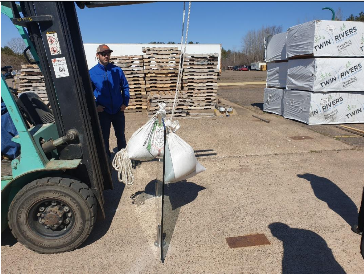
Photo 3: Vertical load test
