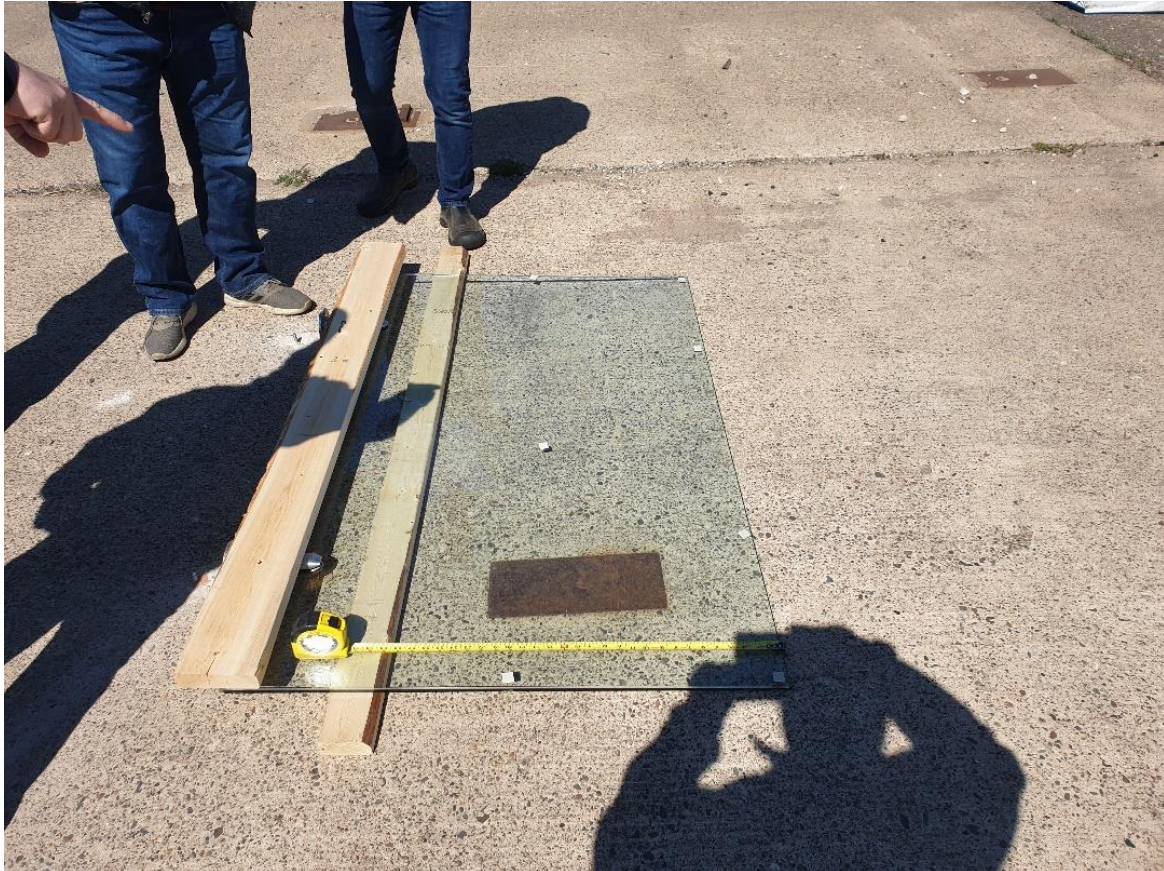
Photo 4: Horizontal load test layout
