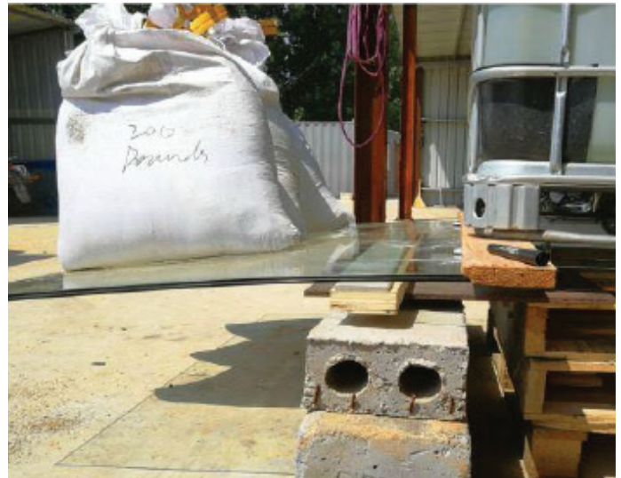
Photo 2: Loading of panel with sandbags, simulating horizontal force
