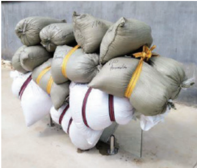
Photo 1: Panel loaded vertically with 2,520 pounds.
