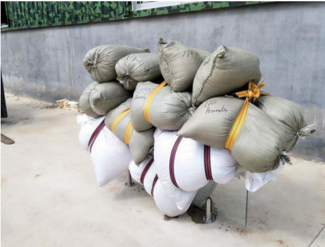
Photo 1: Panel loaded vertically with 2,520 pounds.
