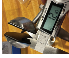
Lever Spigot with shim insert. Shim the opening is approximately 12.9mm.
