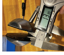
Lever Spigot without shim insert. Shim the opening is approximately 13.9mm.
