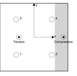
Anchor forces are calculated based on the assumption of a rigid anchor plate.
