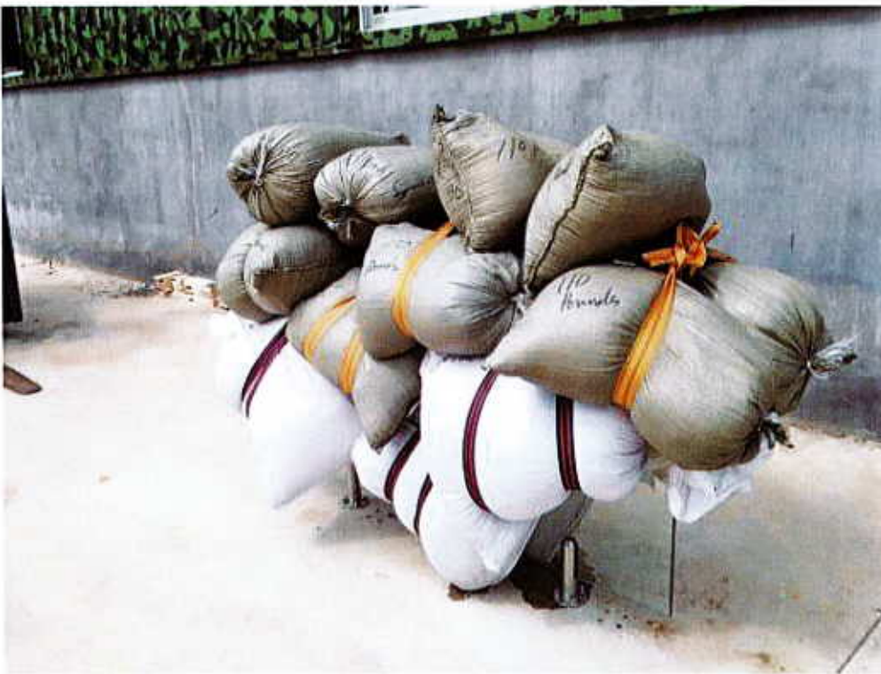
Photo 1: Panel loaded vertically with 2,520 pounds.
